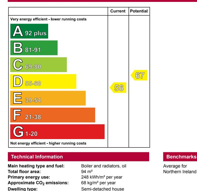
The primary energy use and  $CO_2$  emissions are per square metre of floor area based on fuel use for the heating, ventilation, hot water and lighting systems. The rating can be compared to the benchmark of the average energy efficiency rating for the housing stock in Northern Ireland.
