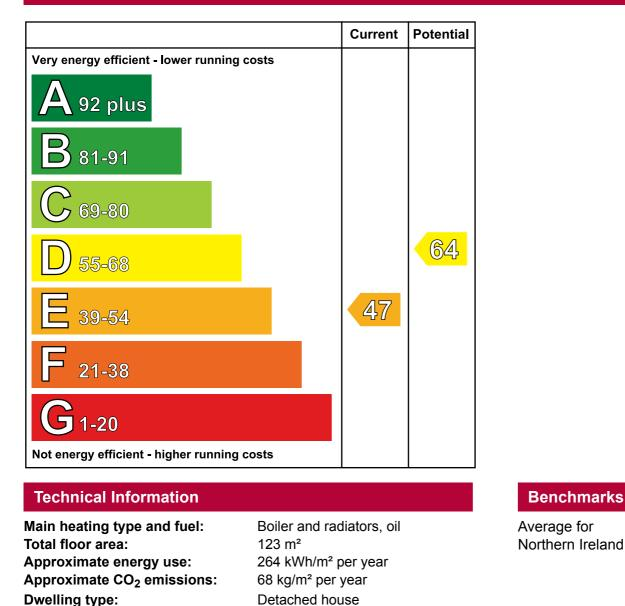
The approximate energy use and  $CO_2$  emissions are per square metre of floor area based on fuel costs for the heating, ventilation, hot water and lighting systems. The rating can be compared to the benchmark of the average energy efficiency rating for the housing stock in Northern Ireland.
